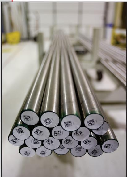
Our drilled barstock thermowells are machined from NACE compliant materials, including 304 and 316 stainless steel, Hastelloy® C276, carbon steel, chrome molybdenum and others. After production, we polish our thermowells to a minimum surface finish of 32 µin R<sub>a</sub> and mark them to ensure material traceability.
